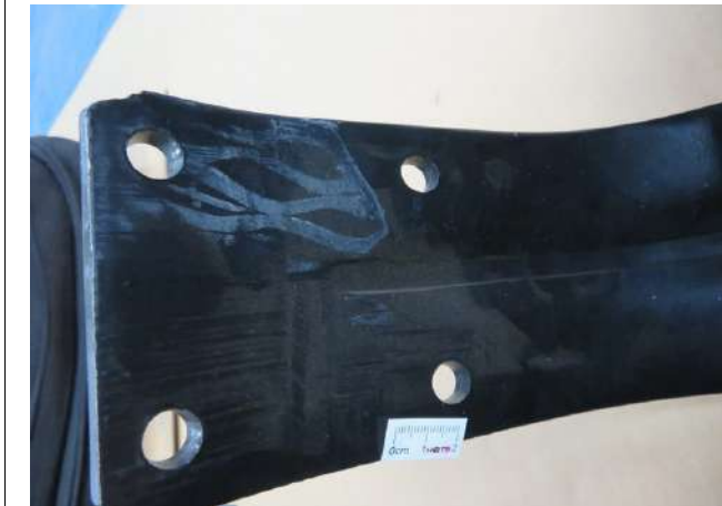
SAP 2.1 Dirty mark at backrest steel surface (can be removed)
