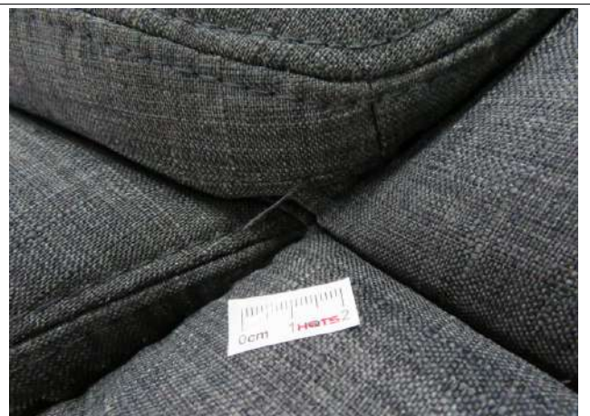
Item 750008-1 Defect-Untrimmed thread end at backrest(1cm)-mi
