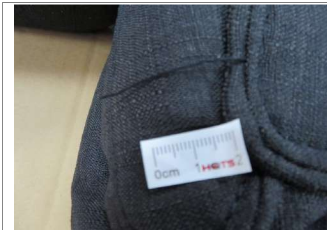
Item 750007-1 Defect-Untrimmed thread end at backrest edge(3cm)-mi
