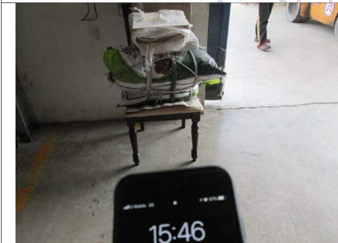
Loading Test #1 (131Kg for 1 Hour)
