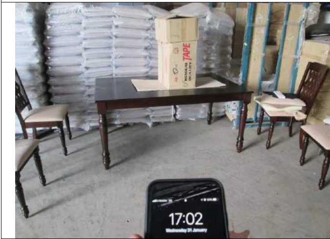
Loading Test #1 (34Kg for 1 Hour)
