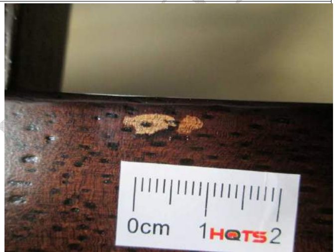
Defect- Improper finishing on Back Leg. (Minor).
