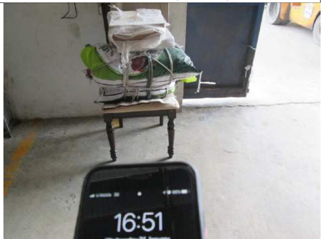
Loading Test #2 (131Kg for 1 Hour)
