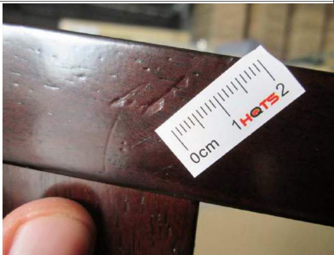
Defect-Dent on Backrest. (Minor).
