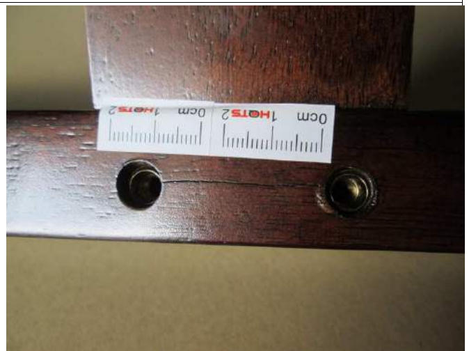
Defect- Crack on Back Leg. (Major). (P2)
