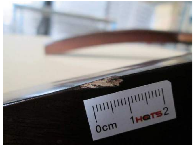
Defect- Chip-off on Back Leg. (Minor).
